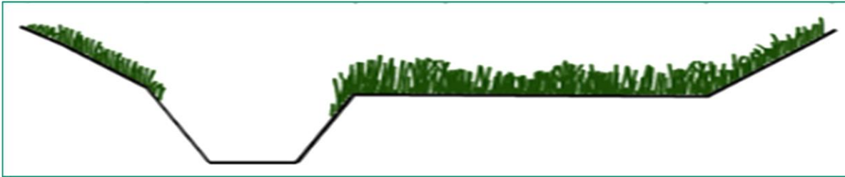
Figure 5.2 – Indicative lowering of right-hand bank (looking in a downstream direction) creating a two stage channel
