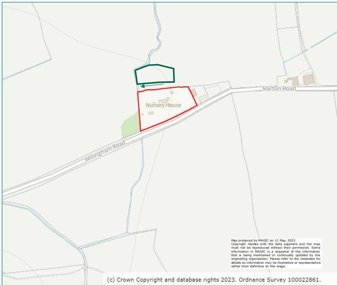
Figure 5.1 – Indicative area to north to lower/reprofile and reconnect existing ditch using open feature (arrow)
